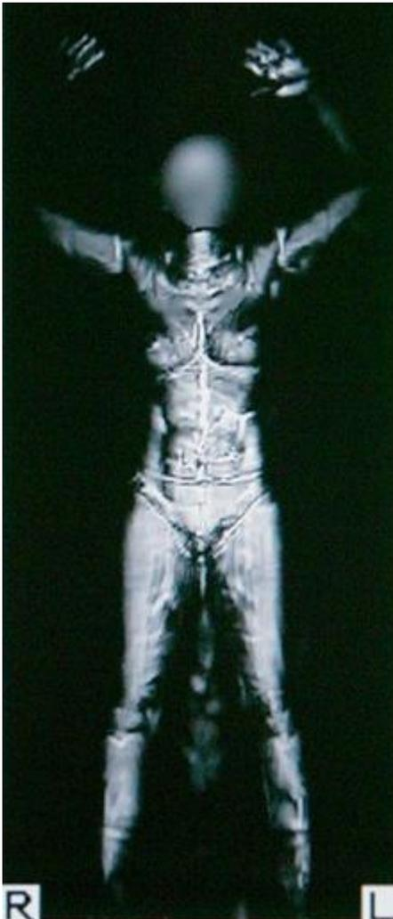
effect of X-rays, a form of ionising radiation. Unlike a traditional X-ray machine which relies on the transmission of X-rays through the object, backscatter X-ray detects the radiation that reflects from the object and forms an image.
